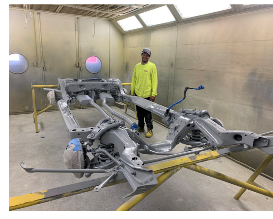
Old car chassis, blasted and primed
