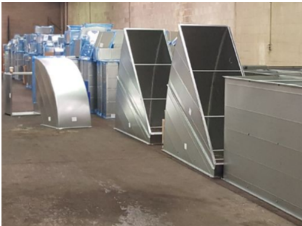
Fabricated Custom Fit Galvanized Duct Work
