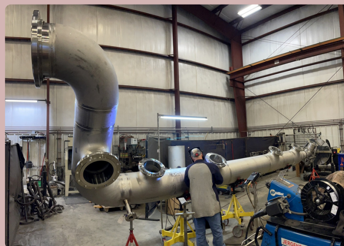
Stainless Steel Brine Main Header
